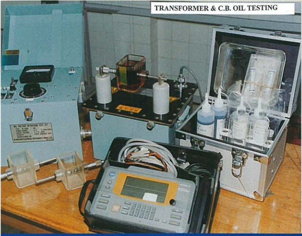
TRANSFORMER & C.B. OIL TESTING
