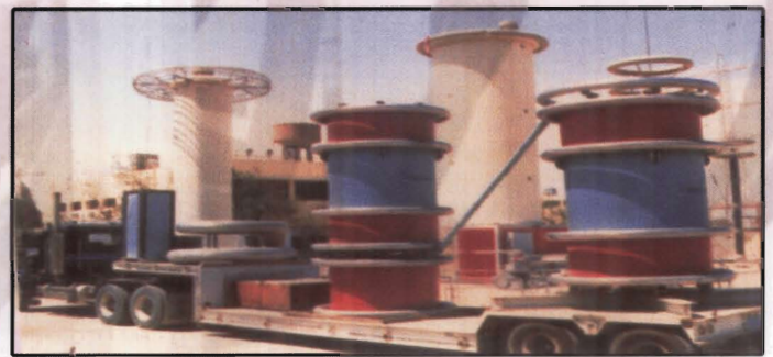
Fig (14) Mobile GIS Testing Facility 800 KV
