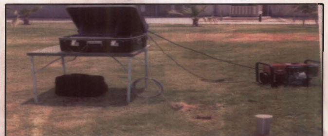
Fig (18) Thermal Soil Resistivity Measuring Instrument
